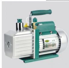
?????? ????? REFCO ECO-3 Technical Data: Free air displacement: 3.0 cfm Number of stages: 2 Microns: 25 Intake threads: 1/4" SAE Flare Motor: 1/3 horsepower Voltage: 115 Volt, 60 Hz Power cord length: 78" Oil capacity: 8 oz / 0.5 pt.
